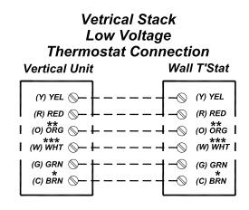
\* - Some thermostats do not use a "C" terminal \*\* - (O) Used in Heat Pump Only
