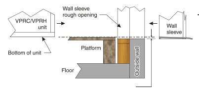
Platform surface must be  $\frac{1}{2}$  inch (13 mm) **ABOVE** bottom of wall sleeve rough opening.
