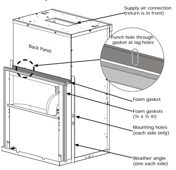
Punch holes in foam gaskets at locations of mounting holes in back panel and weather angles (see call outs in Figure 13 and Figure 14).
