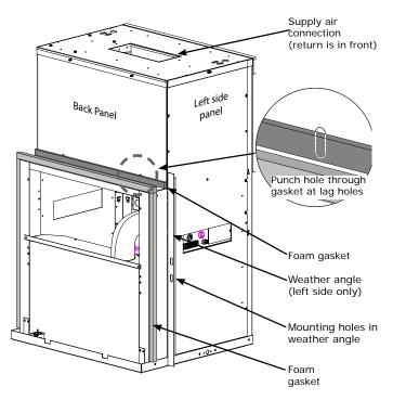
Punch holes in foam gaskets at locations of mounting holes in back panel and weather angles (see call outs in Figure 13 and 14).
