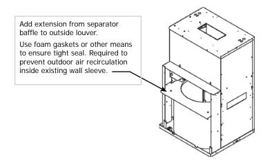
Figure 29 Baffles On Back Of Condenser Coil
