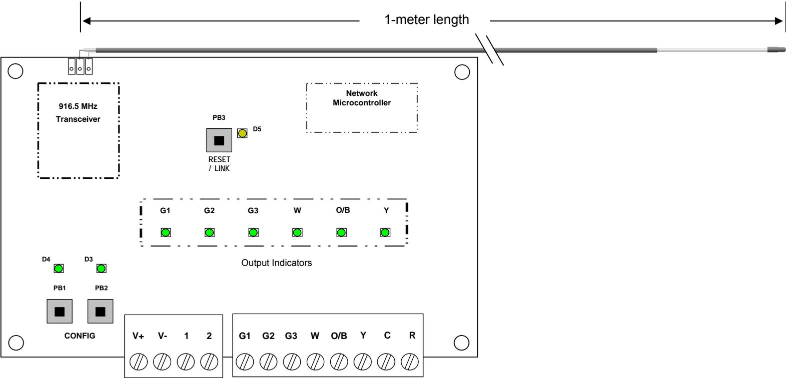
Figure 2 – Model 12200A PCB with Coaxial Antenna
