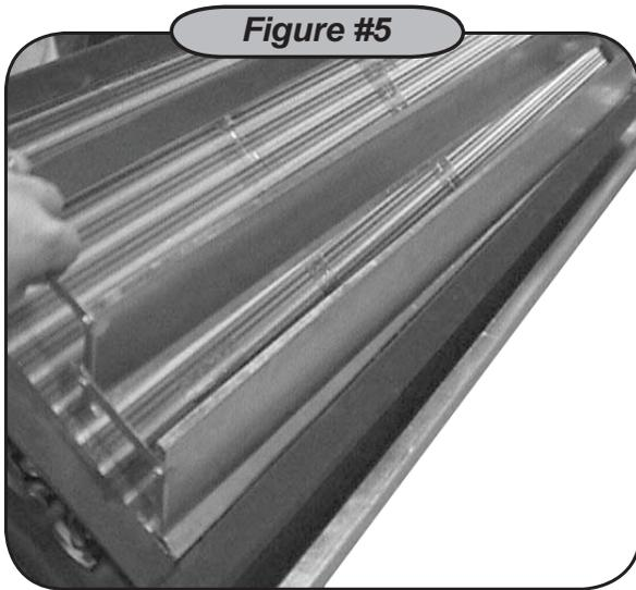
5. Install the mounting brackets to the unused drain pan using 2 - #10 x 3/8" screws supplied. Floor configuration shown.
