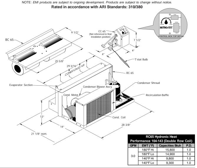
**RC65 ELECTRICAL SPECIFICATIONS** EVAP FAN COND FAN COMPRESSOR TOTAL **MIN** MODEL# VOLTS/HZ/PH M.C.A. RLA AMPS AMPS ΗP LRA ΗP AMPS VOLT 115/60/1 2.5 1.4 0.08 11.3 104 13.2 0.17 7<u>.4</u> 44 9 208/230/60/1 1.1 0.15 3.8 20 0.6 0.08 5.5 197 6.5 115/60/1 2.5 0.17 9.7 54 1.4 0.08 13.6 104 16.0 12 208/230/60/1 1.1 0.15 4.8 26.3 0.6 0.08 6.5 197 7.7
