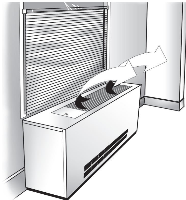
Figure 32 Proper Air Flow Example
