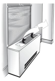
To ensure optimum performance of your PTAC/ PTHP, avoid restricting the air flow. The position of curtains or drapes over supply air grille may cause air to recirculate without cooling the room. The unit will short cycle and may cause premature compressor failure (see Figure 8).
