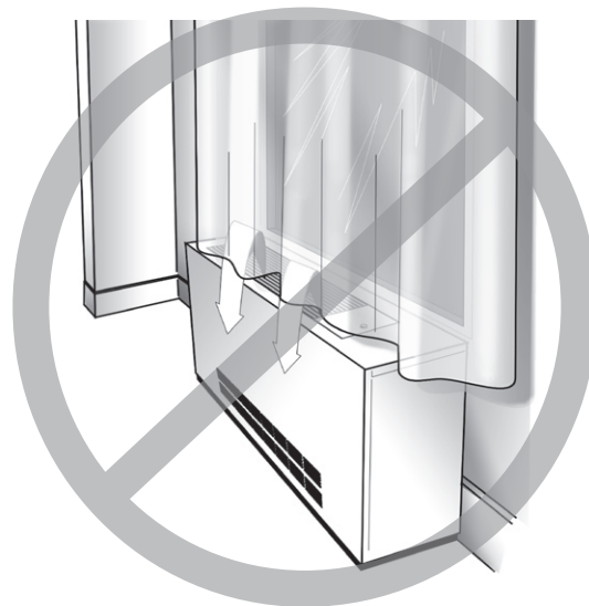
Figure 9 Restricted air flow diagram
