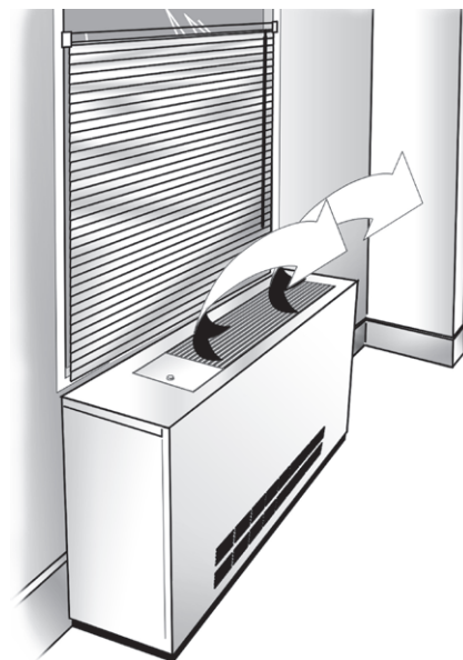
Figure 8 Proper air flow diagram
