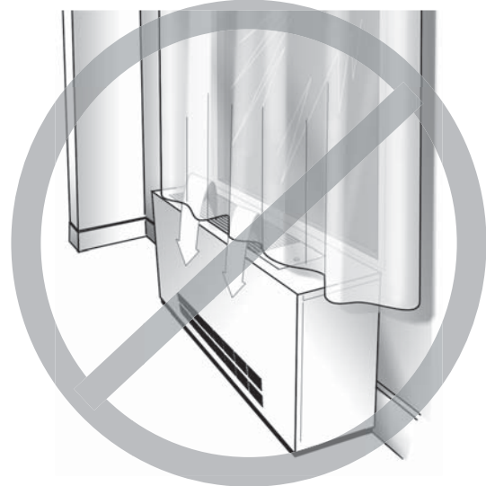
Figure 29 Restricted air flow diagram
