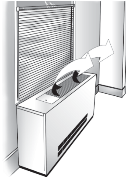
Figure 28 Proper air flow diagram
