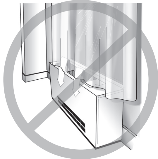
Figure 33 Restricted air flow diagram
