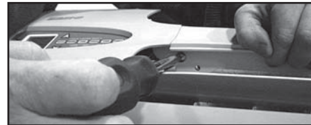
Figure 16 - Rotate Louver Down To Expose Screw
