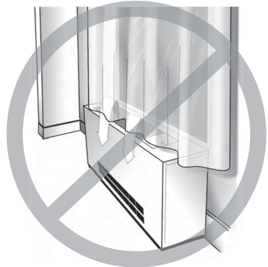
Figure 9 Restricted air flow diagram
