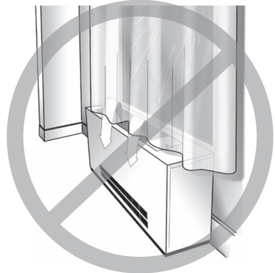
Figure 7 Restricted air flow diagram
