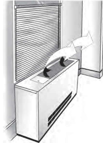
Figure 29 Proper air flow diagram
