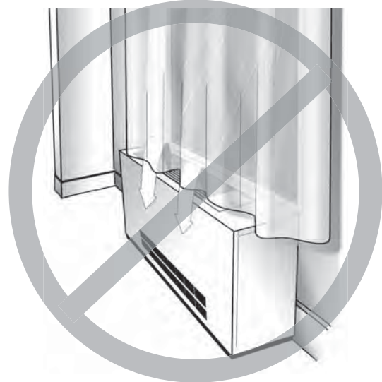
Figure 30 Restricted air flow diagram
