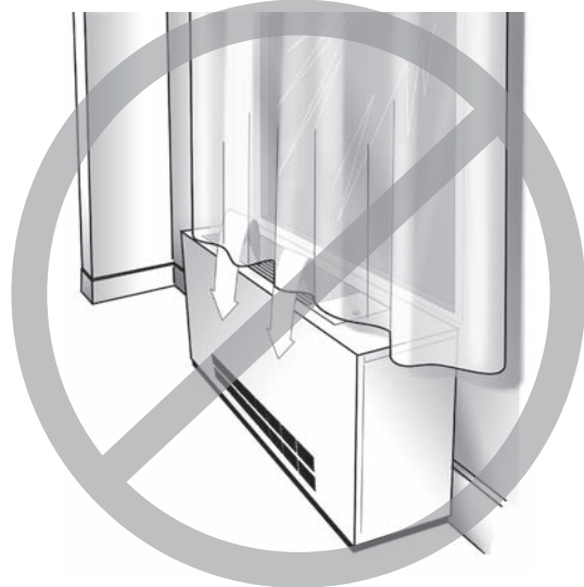
Figure 40 Restricted air flow diagram
