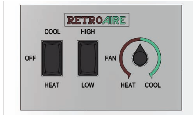
Figure 12 Typical Representation of a Unit Mount Control
