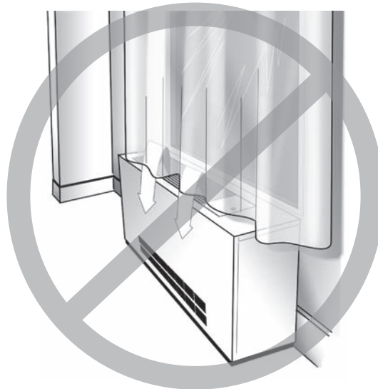
Figure 11 Restricted air flow diagram
