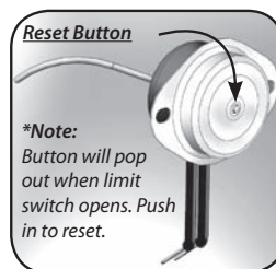
Figure 38 Manual Reset Limit Switch
