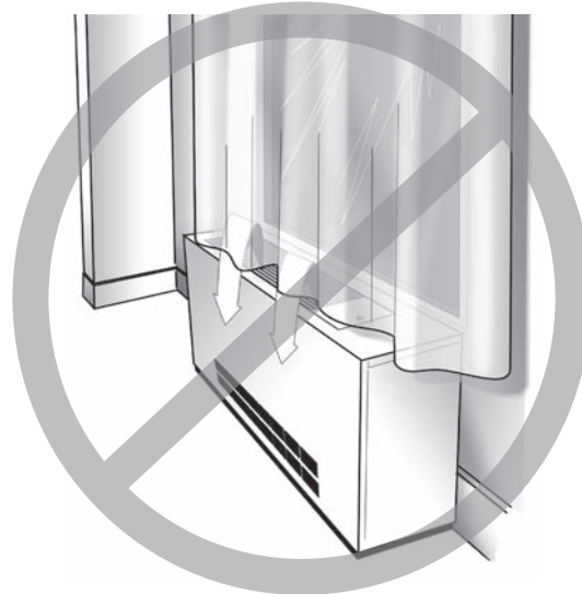
Figure 33 Restricted air flow diagram
