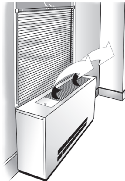
Figure 32 Proper air flow diagram
