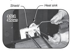
The use of a heat shield is recommended to protect the paint. (A heat shield can be made from scrap metal.)
