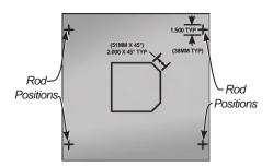
**NOTE:** Make sure the ceiling grid is supported separately from the Cassette. The ceiling must not be supported by any part of the Cassette unit, fascia or any associated wiring or pipe work.
