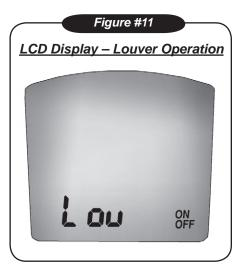
In Cooling, Heating, Auto changeover or Fan Modes, when the louver is on, the louver will oscillate continuously. When the louver is off, the louver will remain in a fixed position.
