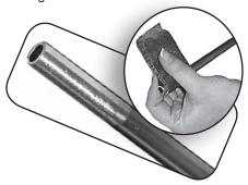
2. Protect the valves by wrapping with a wet rag "heat sink" before brazing.
