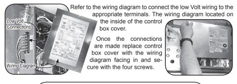
**NOTE:** All low volt interconnect wiring must be at least 18 AWG.
