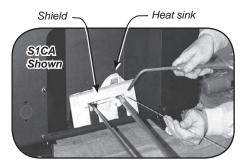
3. The use of a heat shield is recommended to protect the paint. (A heat shield can be made from scrap metal.)
