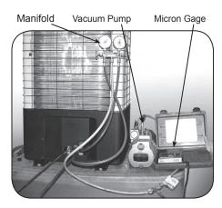
Evacuate line to 500 microns or less to ensure all moisture has been removed and there are no leaks.
