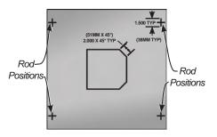
**NOTE:** Make sure the ceiling grid is supported separately from the Cassette. The ceiling must not be supported by any part of the Cassette unit, fascia or any associated wiring or pipe work.
