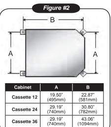
A template for ceiling cut-out and rod positions can be found with the Cassette unit.
