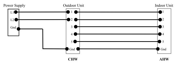
NOTE: Gnd is Earth Ground ACW is cooling only indoor unit CCW is cooling only outdoor unit AHW is heat pump indoor unit
